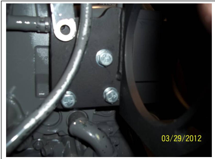
Compressor mount fastened to engine with three M10 bolts, locks, and flat washers.
