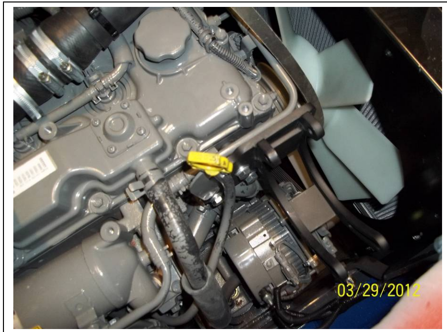
Install the compressor mount with M10 bolts, locks and flat washers provided. Check vertical alignment and tighten in place. Some careful bending on the dip stick tube will bring it in closer to the engine. Do not bolt it to the bracket yet.
